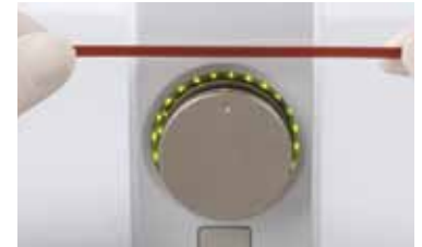
Ready LED ring indicates device status
